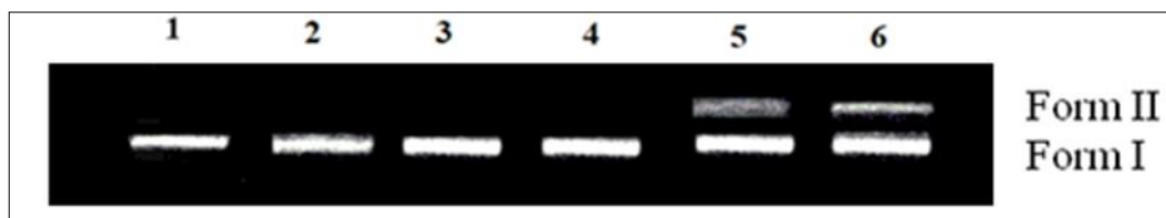
Fig 8.(a). The metal complexes oxidatively cleaved supercoiled pBR322 DNA (0.2 \mu g, 33.3 \mu M) at 37 °C in a buffer of 5 mM Tris HCl/5 mM NaCl. 1 st lane, DNA control; 2 nd lane, DNA + H 2 O 2 (1 mM); 3 rd lane, DNA + H 2 O 2 (1 mM) + HL 1 ; 4 th lane, contains DNA + H 2 O 2 +HL 2 ; 5 th lane contains DNA + H 2 O 2 (1 mM) + 1a; 6 th lane, contains DNA + H 2 O 2 (1 mM) + 2a.
