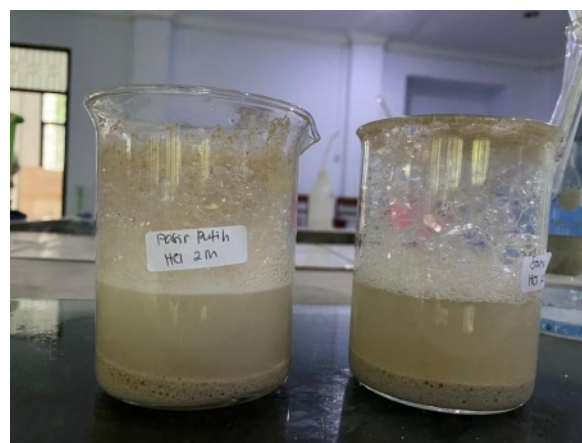
Fig 1: Process of soaking sand with HCl (a) soaking sand with HCl at a concentration of 2M
